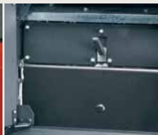
Pulizia tubi caldaia Boiler tubes cleaning Nettoyage tuyaux chaudière Kesselrohre Reinigung
